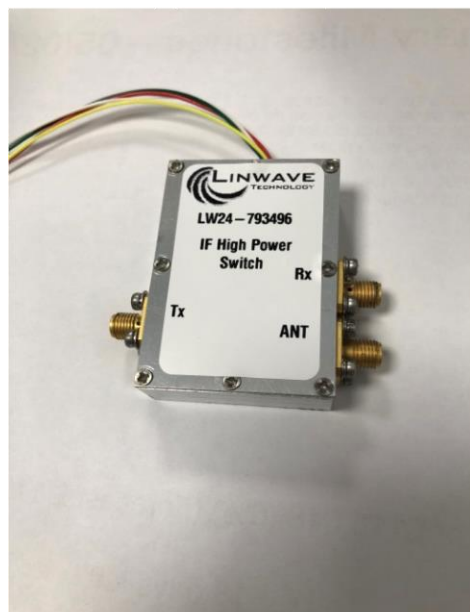
Figure 1. TX / RX Switch
