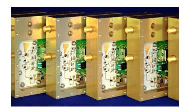
The designs are full SMT allowing for low cost high volume manufacturing techniques. An internal 10MHz reference can also be included as an option. The frequency converters can be supplied as single units to be integrated into bigger amplifier systems or fully weatherised for outdoor use with optional integral mains power supplies.
