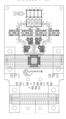
The circuit board used in the application should use RF circuit design techniques. The signal lines should have 50 ohms impedance and the package ground leads and package bottom should be connected directly to the ground plane similar to that shown. A sufficient number of via holes should be used to connect the top and bottom ground planes. The evaluation circuit board shown is available from Linwave upon request.
